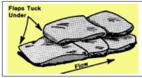
Place the sandbags to form a pyramid by alternating header courses (bags placed crosswise) and stretcher courses (bags placed lengthwise).
